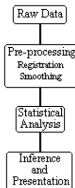
Figure 6.1 Steps involved in the processing of fMRI data
