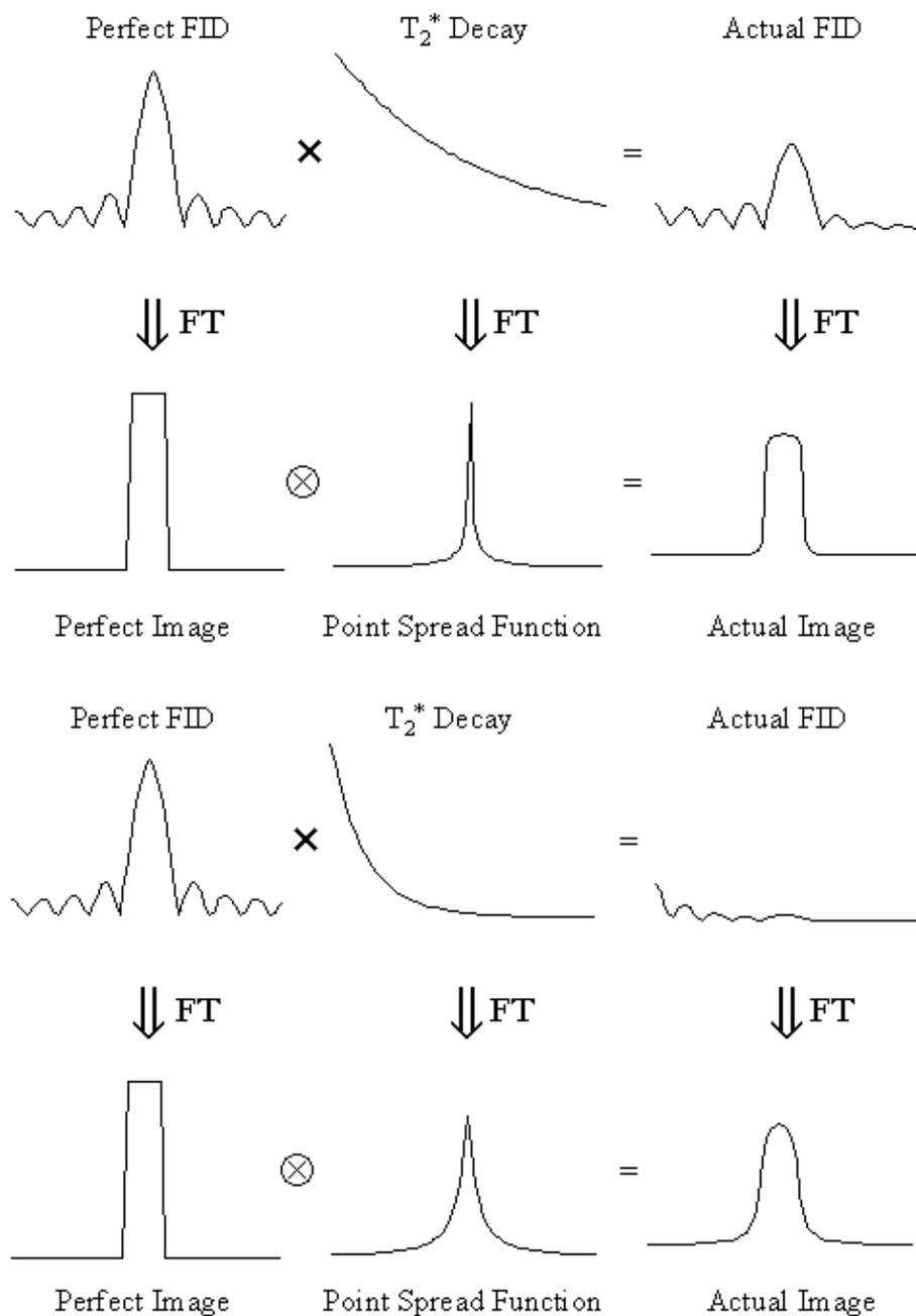
**Figure 5.9** The effect of  $T_2^*$  decay on the sharpness of a line through an image. The smaller the value of  $T_2^*$ , the wider the point spread function, and the more smoothed the profile becomes.
