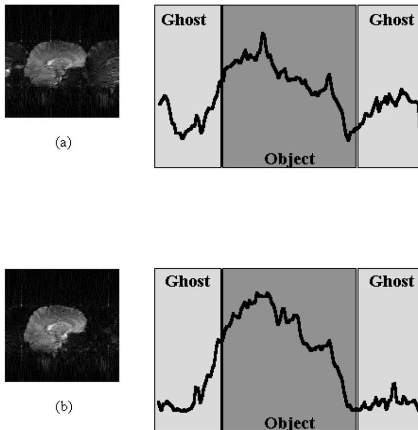
**Figure 5.12** Profile of Fourier Transform of the central line of k-space for two shot interleaved EPI images, (a) with severe ghosting and (b) with little ghosting. The ratio of the central lines of this profile to the outside lines is a maximum for a ghost free image.
