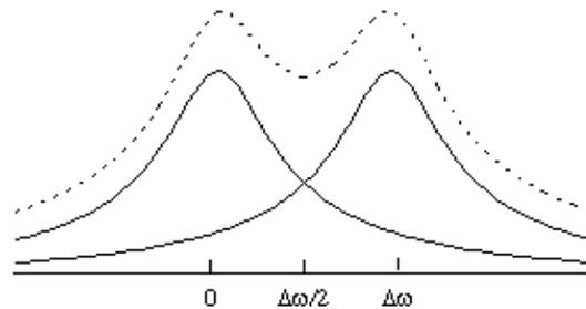
**Figure 5.10.** The Rayleigh criterion applied to the resolution of two pixels subject to  $T_2^*$  line broadening. The intensity of the central pixel must be less than 0.81 that of the intensity of the two pixels it separates.
