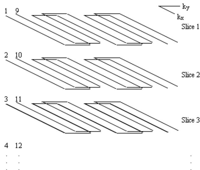
**Figure 5.5. K-Space diagram for multi-slice interleaved EPI.**
