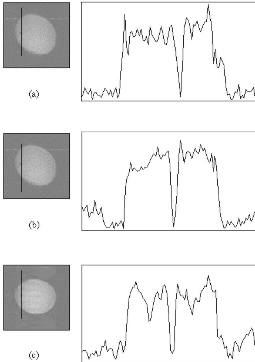
**Figure 5.11** Line profile through a phantom imaged using (a) single shot, (b) two shot and (c) four shot interleaved EPI. The pixel resolution is  $1 \times 1 \text{ mm}^2$  and the glass rod in the phantom has diameter 3 mm. The narrower point spread function, in the broadening direction, of the four shot image means that the rod is better defined than in the single shot case.
