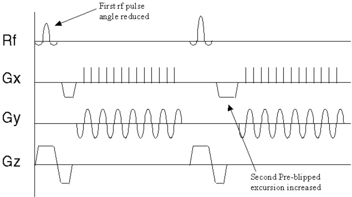
**Figure 5.2. Pulse sequence diagram for a two shot interleaved EPI experiment.**
