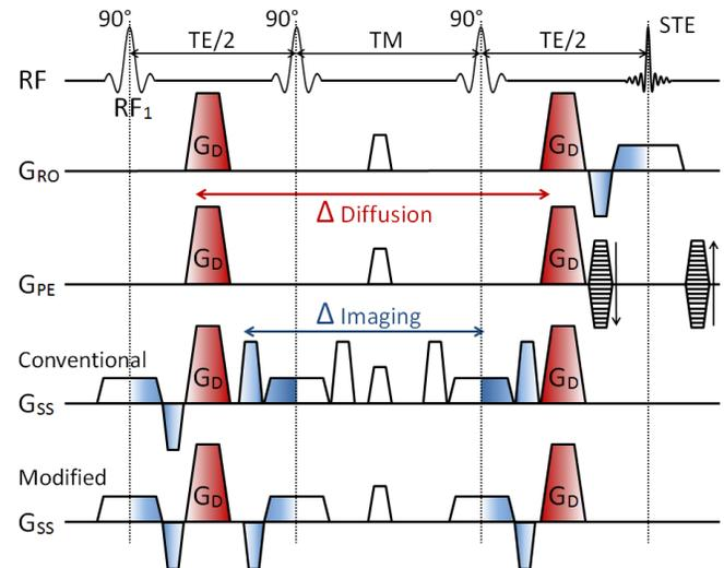
**Fig. 1.** Conventional and modified DW-STE imaging sequence.
